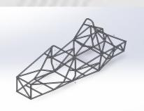
The tubular spaceframe chassis for our Formula Student car was designed in SolidWorks for optimal performance, safety, and manufacturability. Made from lightweight, high-strength BS4 T45 steel, it provides excellent torsional stiffness to handle racing loads. The design, prioritizes driver ergonomics, and complies with Formula Student safety standards. Finite Element Analysis (FEA) validated the structure, ensuring a balance between strength and weight for peak track performance.
