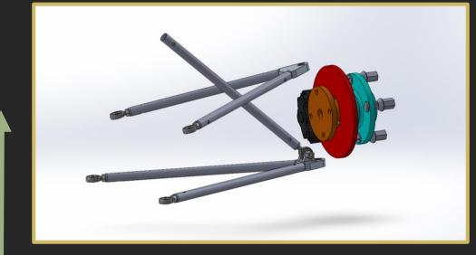
The rough shape of the suspension bracket was designed. Initially the shock absorber mounts were a sperate part.
