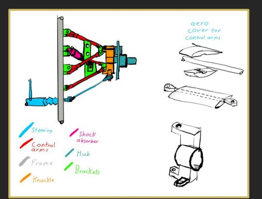
A design for a bracket that will be at the end of the control arms. The control arms are designed to thread in.
