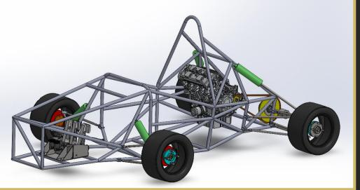
The completed control arms were inserted into the car assembly. The suspension mounts onto the chassis. The suspension design conforms to all completion regulations.
