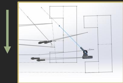
All the components were put into an assembly to check for clearances. Below is the front suspension assembly.
