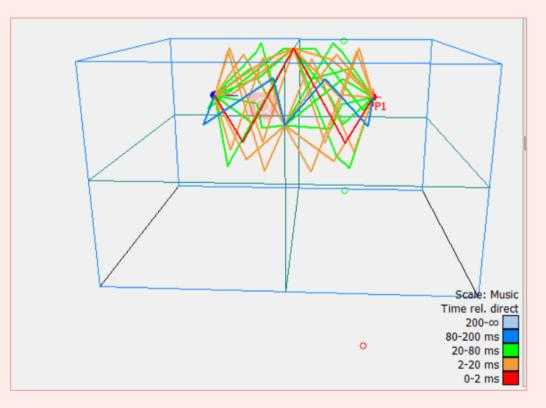
This is one example of how sound travels from the source (P1) to the receivers through walls, floors, and flanking paths. Different colours represent **delay times** for reflected sound energy.
