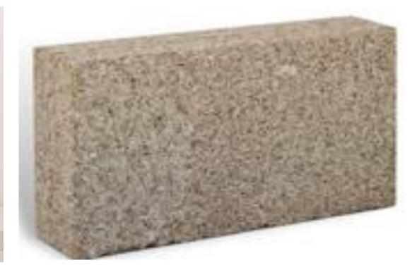
Hempcrete is a mixture of hemp, lime and water. It is then compressed and dried. This material could potentially serve as a future replacement for concrete. It has a lot of favourable properties for construction, such as fire resistance, energy efficient and is naturally nontoxic.
