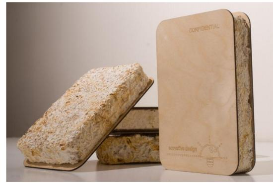
Mycelium Materials are materials that are mainly made out of mycelium. The use of mycelium reduces carbon, and it is also renewable as more mycelium will grow.
