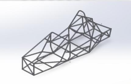
The tubular spaceframe chassis for our Formula Student car was designed in SolidWorks for optimal performance, safety, and manufacturability. Made from lightweight, high-strength BS4 T45 steel, it provides excellent torsional stiffness to handle racing loads. The design, prioritizes driver ergonomics, and complies with Formula Student safety standards. Finite Element Analysis (FEA) validated the structure, ensuring a balance between strength and weight for peak track performance.
