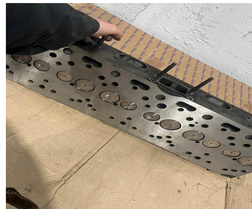
Bottom face of the head that has been skimmed and fitted with new valve:
