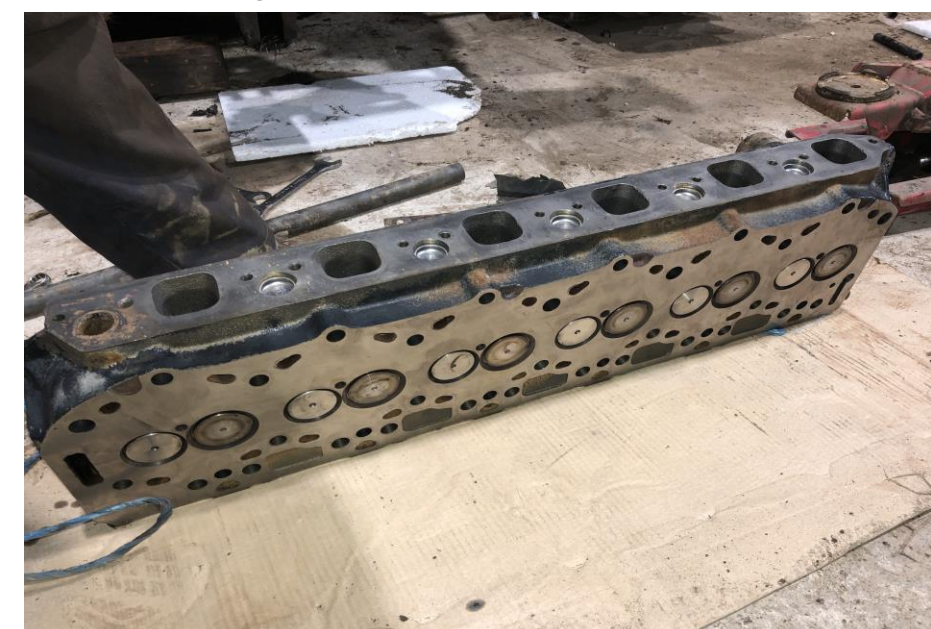
Picture of bottom of engine head after resurfacing
