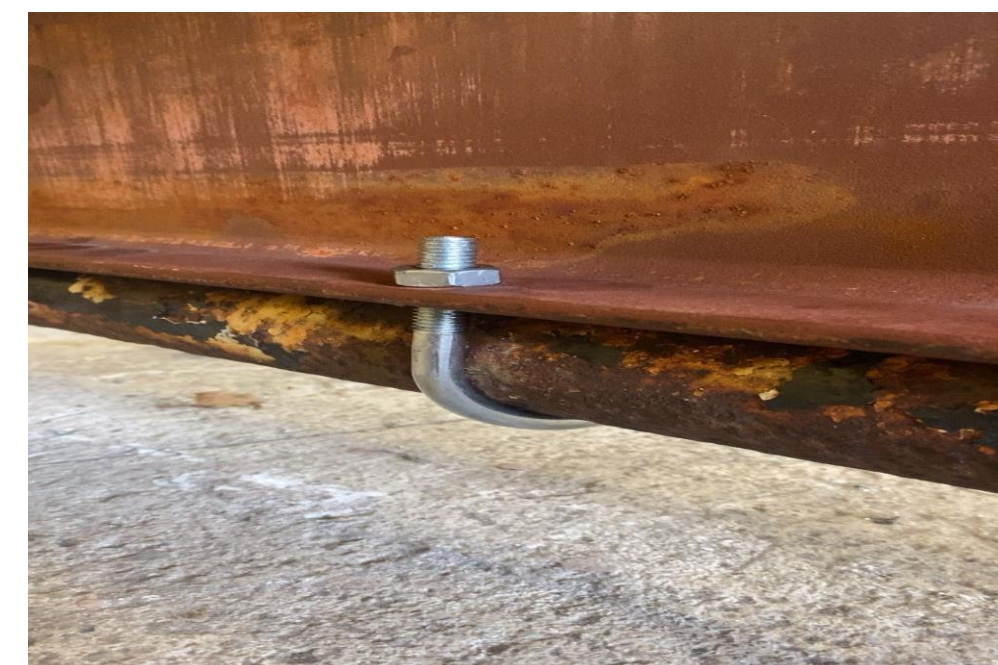
Picture illustrating how I mounted the RSJ to the drawbar using U-bolts
