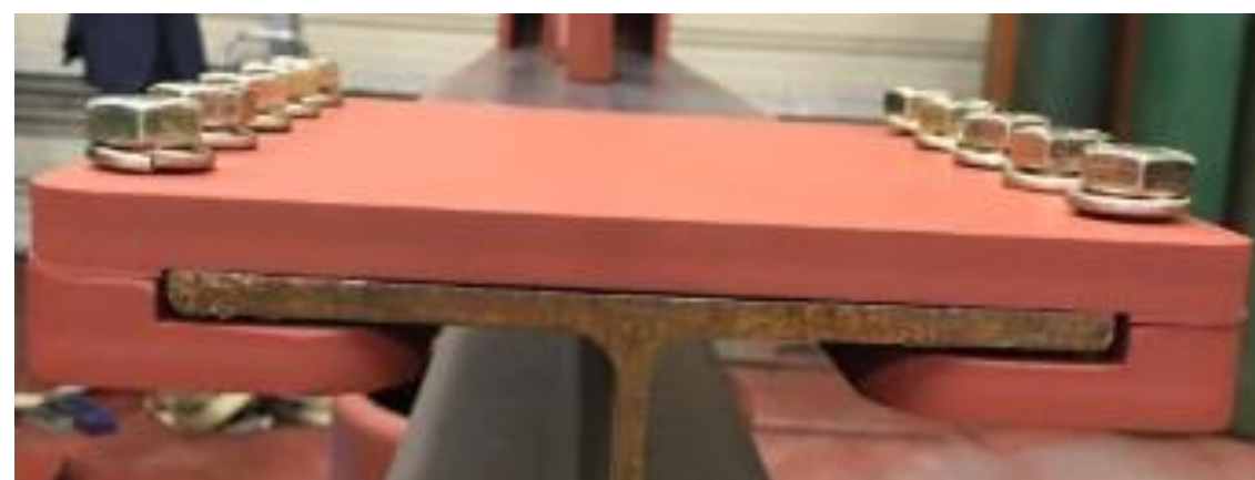
Push plate mechanism I based mine on with bolts to reduce play on the plate
