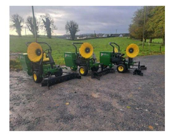
The machines shown in the picture are similar to what my machine will be once it is finished. These machines help to speed up the process of scraping and liming cubicles as they are a lot faster and more efficient than a hand scraper and brush.
