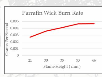
We conducted a calorimetry experiment to measure the heat energy released by paraffin. The experiment found the optimal height to be 55mm which released 128.99 Joules per second of useful heat energy. The final specifications for our engine design can be seen bellow
