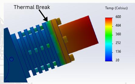
The Thermal Study above was conducted in Solidworks simulation for an 8mm PTFE thermal break. The study illustrated the insulating effects of a thermal break between the hot end cap and hot piston cylinder.
