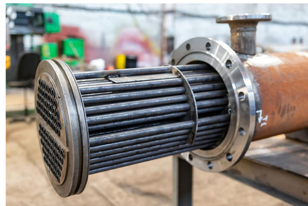
Figure 3: The internals of a shell and tube heat exchanger.
