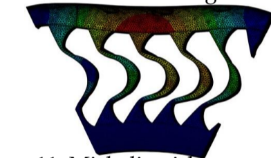
Figure 11: Michelin airless tyre section
