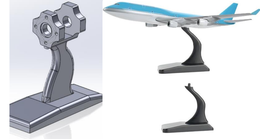
Figure: Initial stand design (left) Model Aircraft stand (right) The initial stand design included three components, the coupler mount, upright part and the base. The inspiration behind the sleek, aerodynamic look of the stand came from the commonly used design of model aircraft stands.
