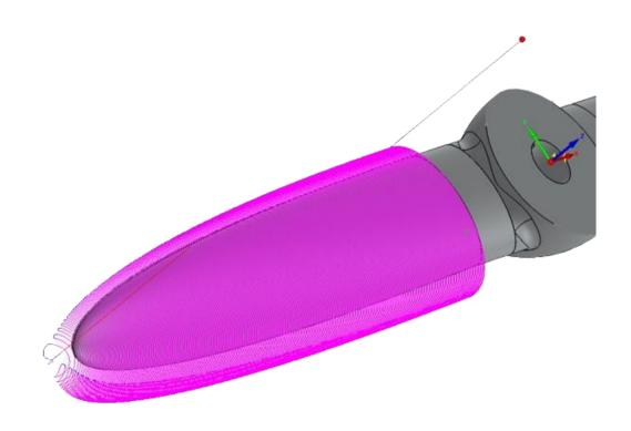
Shown above is the SolidCam toolpath of a HSS finishing pass operation that was done on the blade of one of the propellers.
