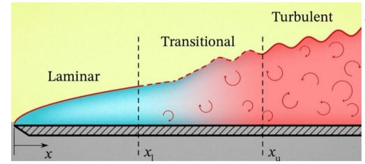
As fluid flows over an object or an object goes through the fluid, the fluid in contact with the object will create a thin layer of fluid moving in a different pattern to that not in contact with the object, depending on the relative velocity the boundary layer will have an increased or decreased Reynolds number which means that the fluid could go from laminar to turbulent flow at a certain distance away from the start of the object
