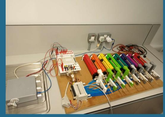
The assembled control box is plugged into the PLC of the pneumatic xylophone. First simple songs were played at 90 beats per minute (BPM). Further tests were conducted with more complex songs and the BPM was increased to 130 BPM. Different songs were uploaded and played. This was done to find what are the best sounding songs to fill up the 12-song playlist
