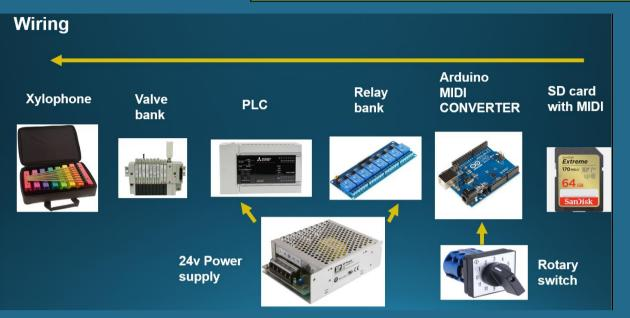
The MIDI files will be on an SD card. This will be converted to output signals that will trigger a relay. The relay signal will be read by a PLC and sent on to a valve bank. The valve bank controls air cylinders that actuate beaters that play the xylophone
