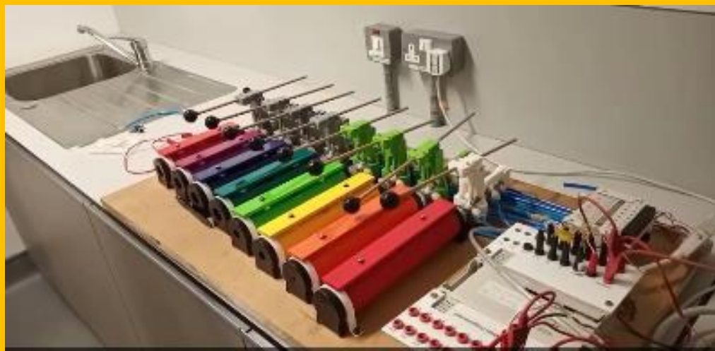
Figure 1: pneumatic-operated xylophone controlled by PLC
