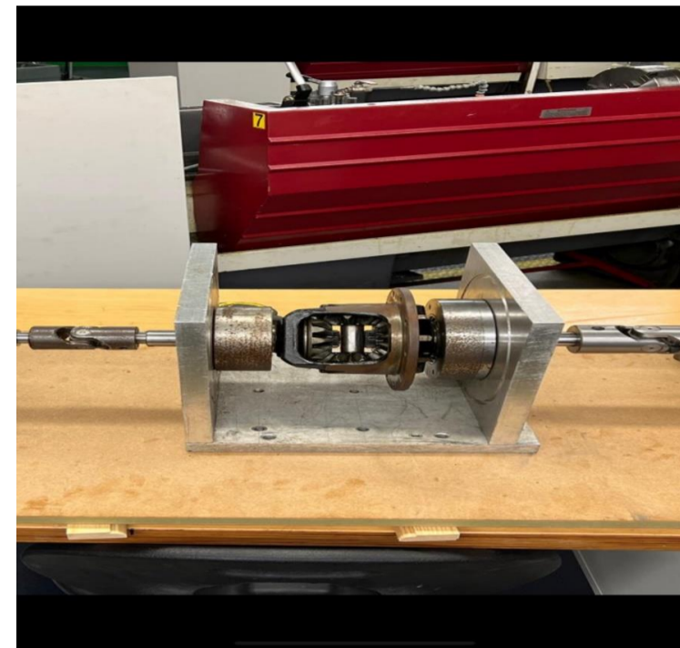
Figure 1: In-line MMR used in prior work
