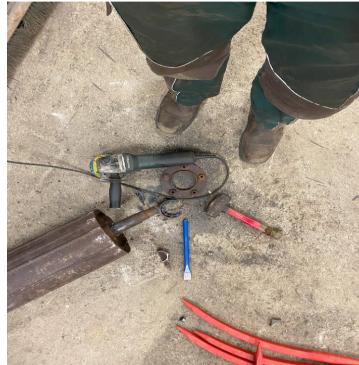
Figure 1: cutting bearing of the roller shaft
