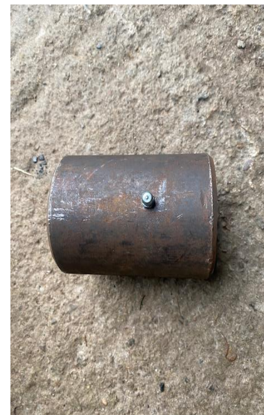
Bushing for 40mm pin with grease nipple
