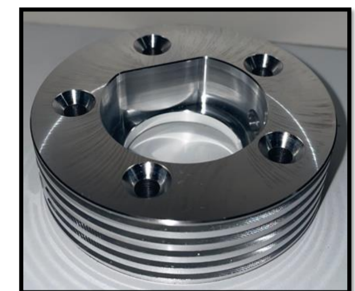
Figure 5- Machined Cylinder Head
