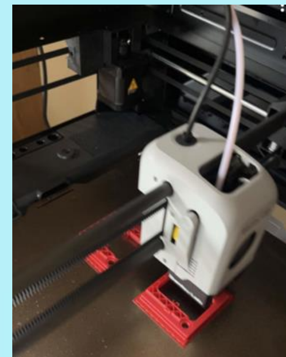
Figure 5 slider being 3D Printed
