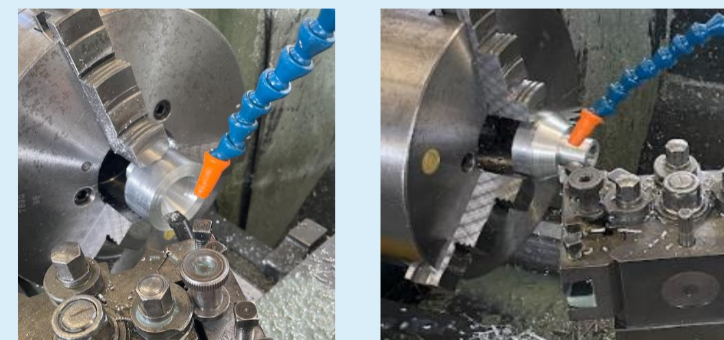
Figure 5 & 6: internal and external machining processes for inlet cone.
