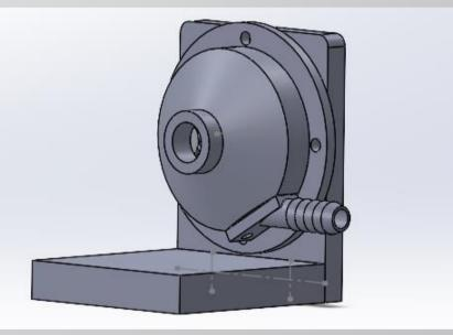
Figure 3: SolidWorks Model of Impeller Assembly
