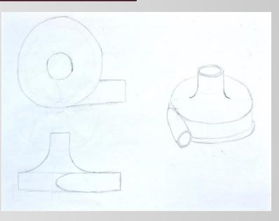
Figure 2: Sketch of Impeller Housing
