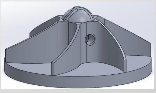
Figure 3: SolidWorks Model of Impeller
