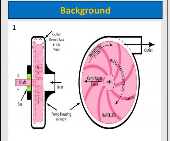
An impeller pump is a type of pump that uses a rotating component called an impeller to increase the pressure and flow of a fluid. As the impeller rotates, it creates centrifugal force, pushing the fluid away from the centre and towards the outlet of the pump. This action helps move the fluid through the pump and into the desired system or application.
