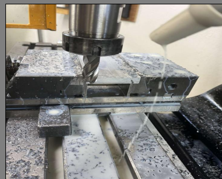
Photo of: Brian milling the base plates
