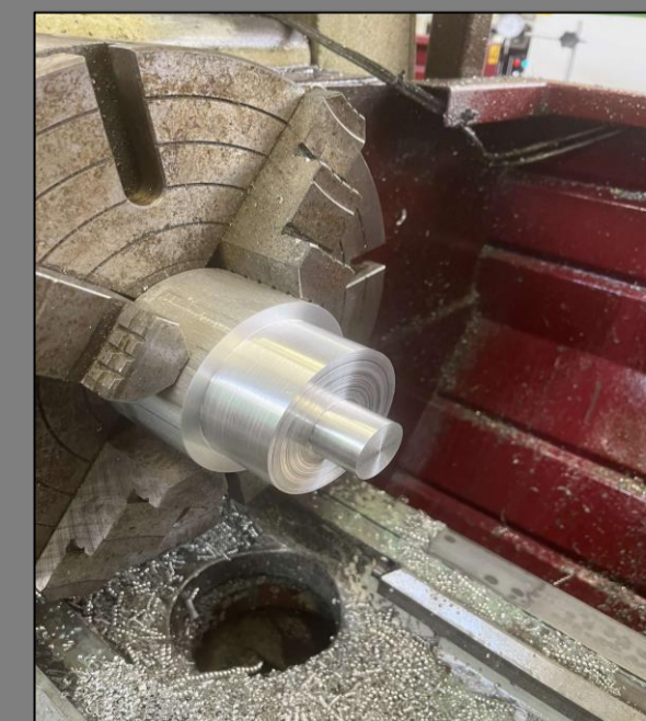
Photo of: Axis piece being machined
