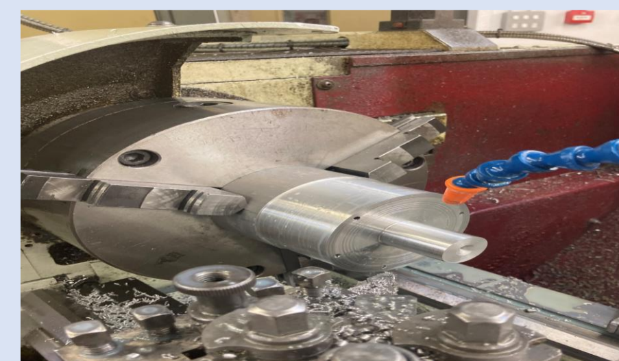
Figure 6: Cutting of outside diameter of Main Casing
