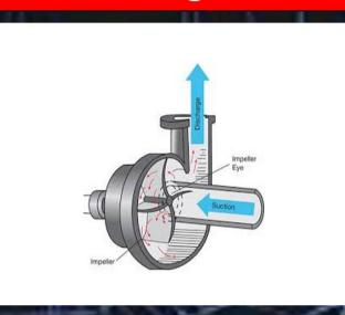
Impeller pumps work off the principle of positive displacement. By turning the impeller creates a region of low pressure at the center of the blade generating suction through the intake and inversely creates a region of high pressure at the periphery of the blade witch in turn produces the discharge
