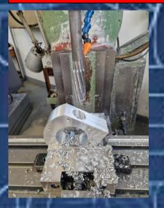
The pump casing had to be mounted at a 30 Deg angle to allow for the boring of the out, angle were used to blocks ensure the correct set up
