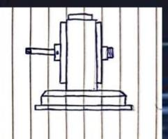
Three concept were produced during the design process. The first design fulfilled the brief the best with the inclusion of the idea of a vertical outlet from the second design to allow for the pump to be primed more easily
