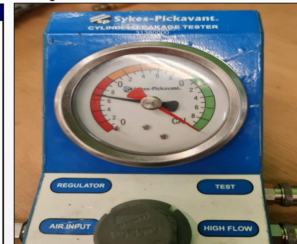
Figure 4: Cylinder leak-down test carried out in the TUS Workshop
